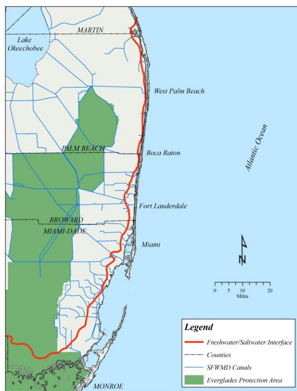
Figure 9.2: Estimated freshwater/saltwater interface in the lower east coast for the years 1995 through 2000 based on measurements from 100 mg/L chloride to 250 mg/L chloride and above. The blue dots indicate the locations of major wellfields for water supply.
